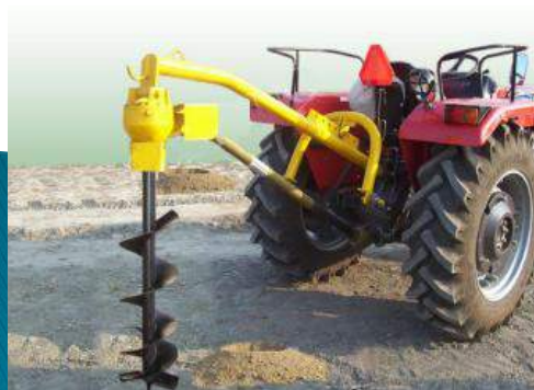
POST HOLE DIGGER
