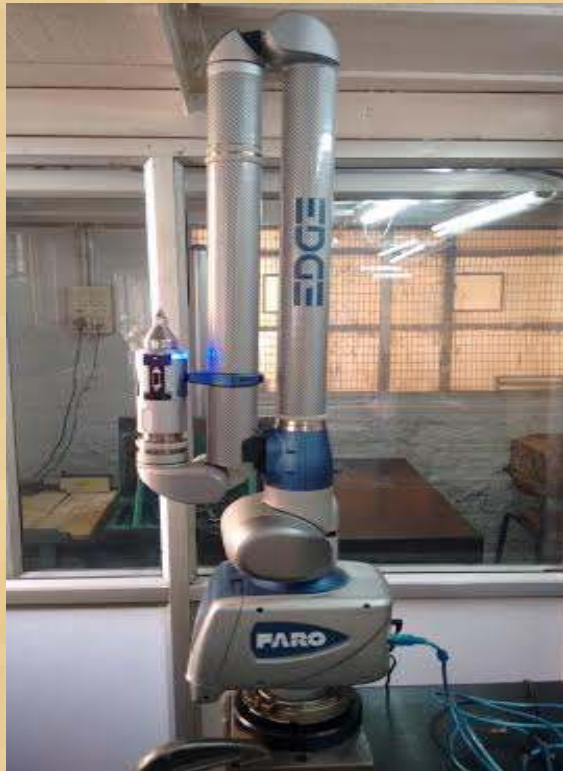
1. FARO EDGE Arm CMM CAM2 Measure 10 Working volume 2.7 meter Single pt Accuracy = 0.029mm Vol. Accuracy= +/- 41 microns
