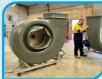
Kitchen Exhaust Blower
