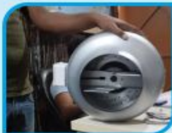
Duct Mounted Fan
