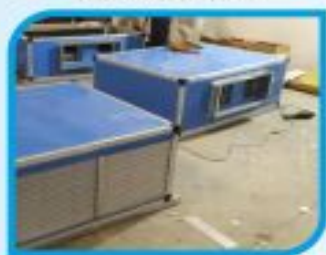
Exhaust Air Units
