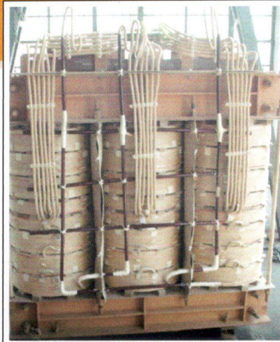
Inner View Of Distribution Transformer
