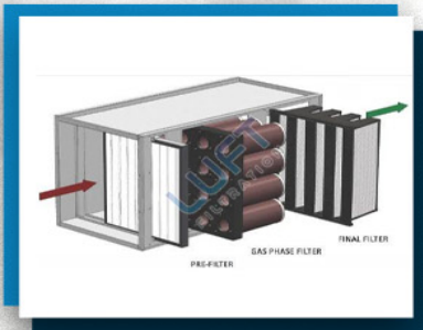
Gas Phase Filtration System
