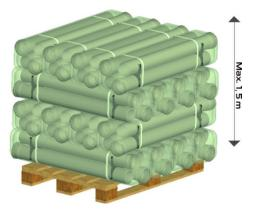
Method of storage should not cause any outflow and should not damage the pipes. As long as they are stored properly, no permanent deformations or damages will occur on the pipes and fittings. Pipes should not be stacked above 1,5 m. Pipes should be safe against sliding. Pipes and fittings packed in carton boxes should be protected against moisture. Carton boxes should be sealed and stored in a dry area.
