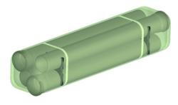
Pipes are packed by plastic clamps to hold them together. Stretch film is applied to protect pipes from pipes dust and stains.
