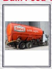
We are engaged in manufacturing, supplying and exporting the best Bulk Feed Tanker. Our Bulk Feed Tanker vehicle is used for carrying the bulk feed or material. Direct loading in bulk feed or materials tanker and unload the bulk feed or materials by tanker conveyors till 35 feet height. With Bulk Feed Tanker, feed millers and customers can save loading, unloading, packing and Ginny bags expenses.
