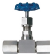
1/8 to 1 Inch Die Forge Body, Union Bonnet with Bakelite Handle or T bar Handle, Different sizes upto 1/2" M & F are available. Material: SS 316 / SS 316 L / SS 304 / CS / BRAS
