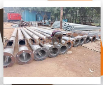
Steel High Mast Pole
