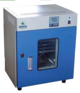
75 mm gap between the walls is filled with special grade glass wool for proper insulation and to avoid heat losses. Inner chamber
