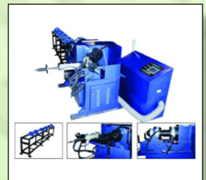
Automatic Pipe And Tube Cutting & Parting
