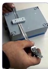
3- Attach the tape to the testing device
