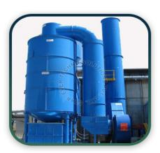
A wet scrubber is a pollution control device used to remove pollutants from industrial exhaust gases or flue gases before they are released into the atmosphere. It operates by using a liquid (usually water) to trap and remove particulate matter and/or gases from the air stream.
