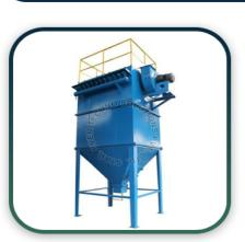
A pulse-jet fabric filter, often referred to as a pulse-jet baghouse, is a type of dust collector that utilizes a cleaning mechanism known as pulse-jet cleaning. This technology is commonly used in industrial applications to remove particulate matter from gas streams, helping to maintain air quality, protect equipment, and comply with environmental regulations.
