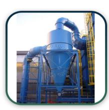
A cyclone separator, often referred to simply as a cyclone, is a device that uses centrifugal force to separate particles from a gas stream. It is commonly employed as a preliminary or primary means of particulate matter removal in various industrial processes.
