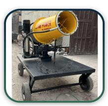
The anti-smog gun is a mobile device that sprays a fine mist of water into the air to reduce particulate matter and pollutants, such as PM2.5 and PM10, that contribute to smog and poor air quality.
