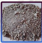
Granulated Blast Furnace Slag (GBFS)
