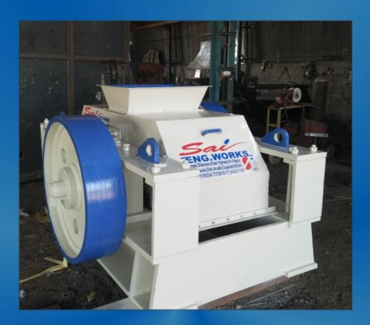
As the material is CRUSHED ONLY ONCE when it passes through the gap, the percentage of FINES IS MUCH LESS.
