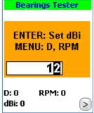
If dbi value is unknown just enter the bearings shaft diameter and RPM and device will calculate the dBi value:
