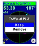
Device displays calculated correction weights to be attached at Planes #1 and #2 to eliminate disbalance.
