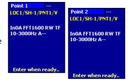
press key. Device takes measurement with preset parameters and saves files to proper destination folder
