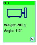
Press to enter trial weight and angle, at which it will be attached
