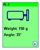
Run the machine and take measure vibration levels at all four points when trial weight is attached at the Plane #2.
