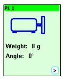
Press to enter trial weight and angle, at which it is attached
