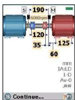
Press - to toggle data input - LD transducer's data / MD - manual data
