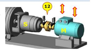
To make adjustment in **horizontal** direction transducers must be turned to 9 or 3 o'clock (90° or 270°) position.
