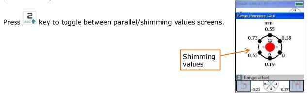
Since transducers are at x45°, 1:30 o'clock (225°) position there is no need to turn shafts to make adjustment in 6-12 plane, just press key to choose which of planes to be adjusted.
