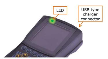
Low flash rate – normal charge, high rate – fast charge. Keep in mind that in most cases PC/laptop USB port can only provide normal charge.
