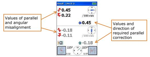
Blue arrows displays directions, in which movable machine must be moved to eliminate parallel misalignment.
