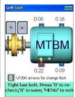
Bolt selection sequence can be changed by manually selecting the bolt by arrow keys.
