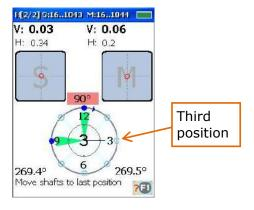
Press to take third reading. When three reading are taken, device will proceed to the result screen. For 4 points mode, one more position should be measured. This mode can be used when advanced alignment precision is required.
