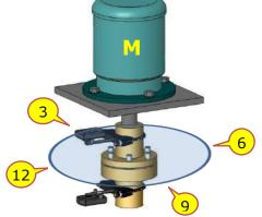
The electronic inclinometers cannot be used on the vertical machines, so "Manual angle" is set by default. One should mark measurement positions on the machine prior to start measuring.
