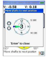
.. and finally turn shafts to the last position
