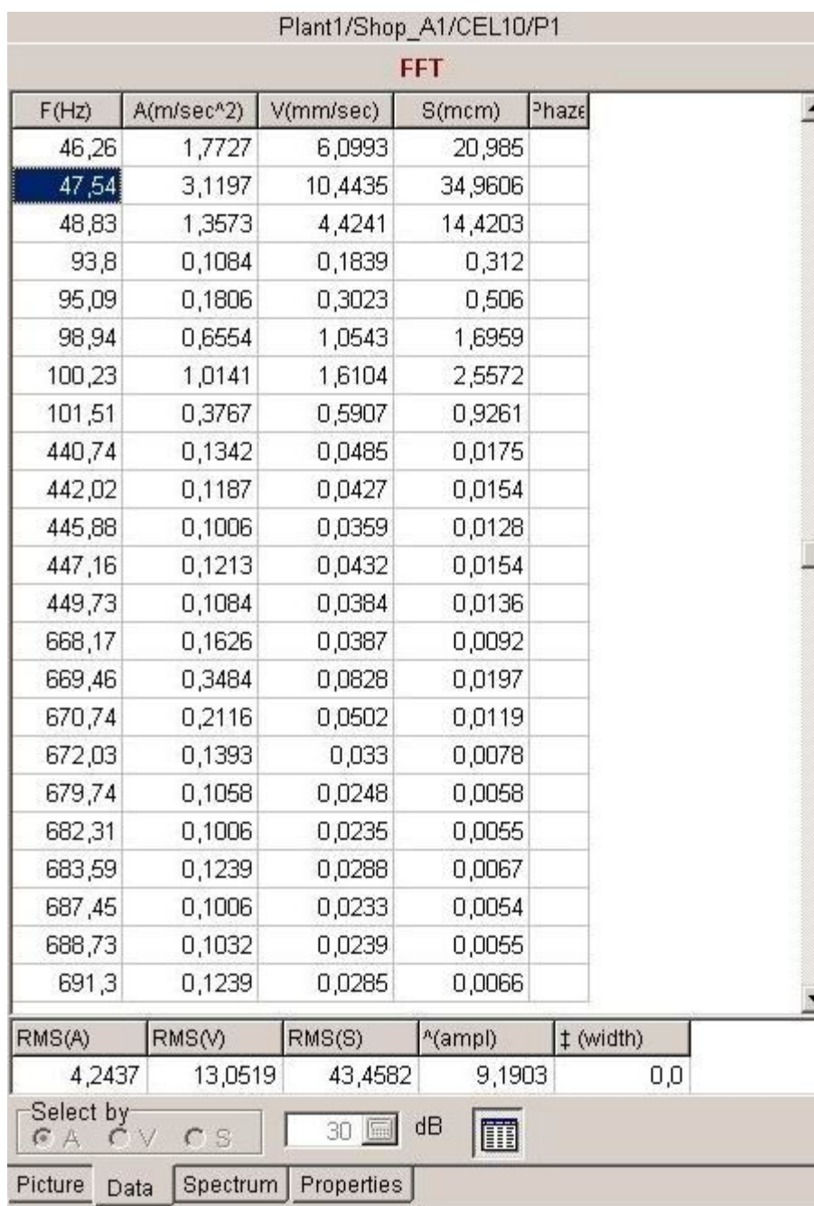
Figure 15 - A bookmark "Data" (the spectrum of vibration is measured)
