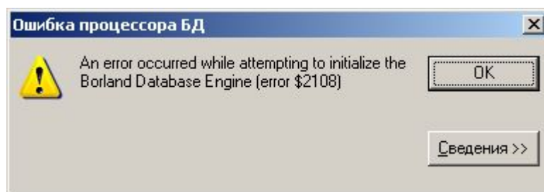
Figure 60 - The message on a mistake at updating the program (it is not established BDE)
