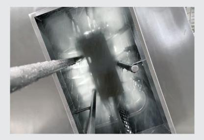
Nozzle units are configured based on milk can size, residue and level of cleaning required
