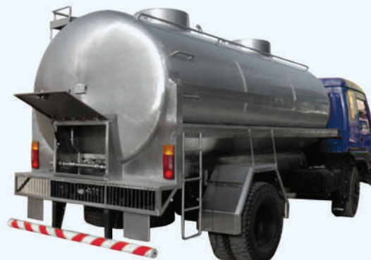
Road Milk Storage Tank
