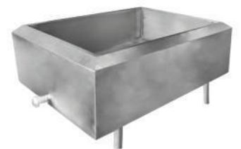
Paneer Coagulation Tank
