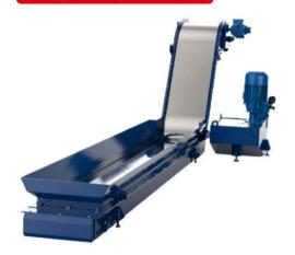
Magnetic chip conveyors are intended for ferrous material applications with small chips. the chips fall on to the conveyors stainless steel surface and are conveyed by powerful magnets moving underneath. The chips are released from the magnetic at the discharge end, and fall freely into a collection container.
