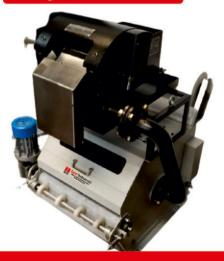
Magnetic coolant filters are designed for filtering coolant oil contaminated with ferrous matrials .the contaminated coolant from the machine is fed into the inlet of magnetic filter. which passes through the gap between the magnetic drum and the body, the drum is driven by a double reduction worm geared motor, the dust particles drum.
