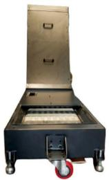
Hinge belt chip conveyors, the most common format, after an effetive means of managionveyorn heavy chip loads and stringy chips. Chips that fall from the machine tool land on the conveyor belt and are conveyed away from the machine tools precision surfaces.
