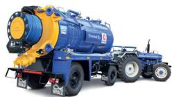
Powerful and multifunctional drain cleaners for simultaneous jetting and suction
