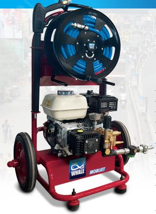
The Mobile Jetting Machine is a high pressure jetting machine for residential and light commercial use. Equipped with a powerful engine and professional pump it is ideal for cleaning walls, floors, ceilings and vehicles.
