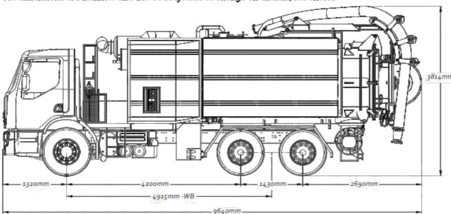
G.A of 25 tonne GVW chassis, call for / ask for 16 tons/ 32 tons
