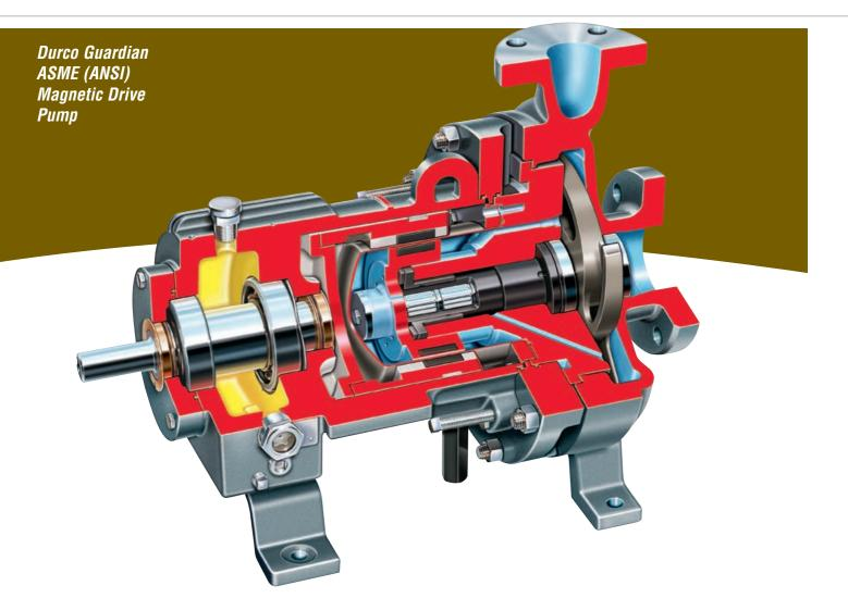
The Flowserve Durco Guardian is a horizontal, magnetic drive pump designed for simplicity and reliability in emission-free services. It is compliant with ASME (ANSI) B73.1-2001 dimensional standards, ASME (ANSI) B73.3-2003 sealless pump standards and HI 5.1-5.6 1992 standards.
