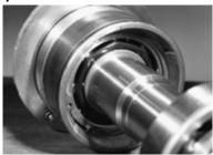
Group 1 and 2 pumps equipped with duplex angular contact bearings use a bearing retainer [2530.1] instead of the snap ring. Remove the carrier from the bearing.
