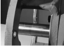
c) Remove the impeller and seal chamber (rear cover) following the instructions given in section 6.7 and install a nose cone onto the end of the shaft.
