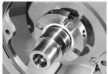
d) Remove the seal or packing gland nuts [6580.2] if so equipped.
