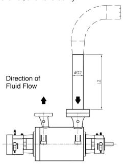
The minimum required straight pipe length (L2) before pump suction inlet is specified in Table 01. The straight pipe section is to be the same diameter as that of the pump section nozzle.
