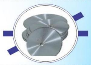
Our Saw Blades are manufactured from rolled steel sheet in Chrome-Vanadium Steel (80CrV2) or 75Cr1. These are called Friction Saws thanks to the friction generated between the teeth of the blade and the working metal. We offer a comprehensive range of dimensions: Diameter up to 1400 mm and thickness up to 10 mm. The blades are provided with uniform hardness.
