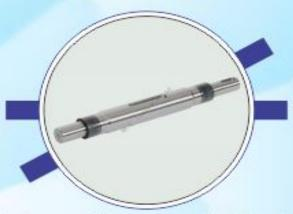
Shafts always support the revolving section of a mill. Since these shafts are subjected to bending, it should have high level of toughness, maximum strength and low stress concentration. To avoid breaking, Case Hardening of these shafts is practiced to maintain a soft core and a hard surface. Grades used are: EN9, EN19, EN24, EN353 and AISI 8620. Provided in various sizes, these shafts are available as:
