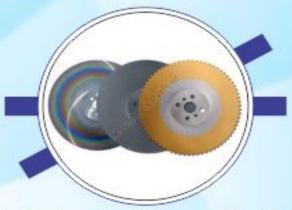
Imported from Japan, these blades are used for cutting steel pipe at a high speed without burr at the ends. HSS Saws are manufactured using High-Speed Steel with a high Molybdenum and Tungsten content improving wear resistance and mechanical endurance. Sizes available are up to a diameter of 500 mm with varied coatings.
