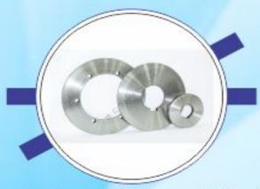
Commonly used grades for Fin Discs are: D2, D3 or EN31. These materials are purposely used because Fins are always under constant wear and high stress due to the strip ends touching them on the periphery before butt welding. Thus, these are provided in hardened and ground state with a uniform hardness throughout. Also, special attention is paid during their heat treatment so that hardened fins are not bent and out of shape.
