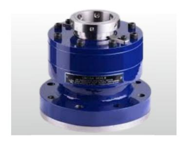
These Cartridge Seaf units are designed for Mixer, Agitators and Glass Lines Recotors. The Heavy duty construction of the 50 seriesprovides long seal life and excellent repairability. The design incorporates bearing located very close to seal. The design specifically is engineered to accommodate the run-out conditions, up to 0.5mm. Large clearance between ration shaft/ sleeve and mating ring permits higher deflection of the shaft.
