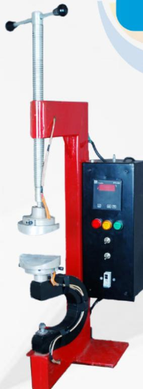
Tyre cut repair machine, also known as a tire vulcanizer or spotter, is a piece of equipment used to repair large, damaged sections of vehicle tires. These machines use a process of heat, pressure, and special rubber materials to permanently bond a patch over the cut, restoring the tire's structural integrity.
