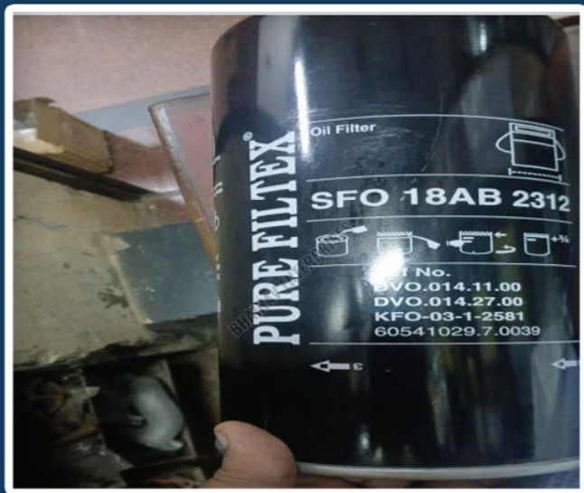
Diesel Engine Fuel Oil Filter
