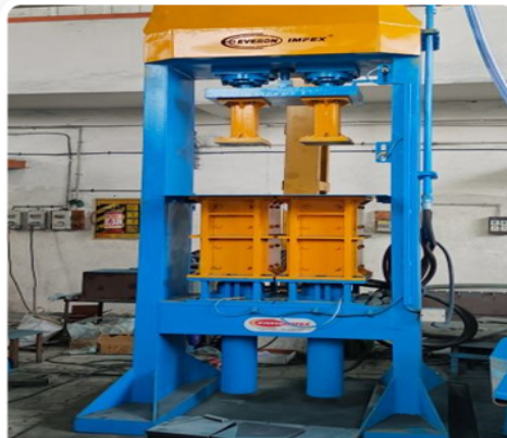
Mild Steel Mud Block Machine
