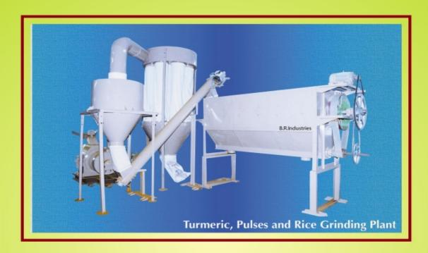
Consists of 1 No. of Cone Type Pulveriser (Grinder) Grinding all Non abrasive materials upto 300 Mesh. 1Nos Of Screw Conveyor (material lifting from machine to Dresser) and Dresser designed to suit Nylon and steel sieves of different Mesh. Thorough sieving and excellent grading. Plant is Suitable for Turmeric, Urad Dhall, Besan, Dry Ginger, Saw Dust, Coconut Shell, Pharmaceuticals, Chemicals, minerals.
