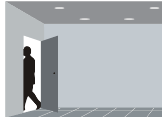
No presence detected, lights off
