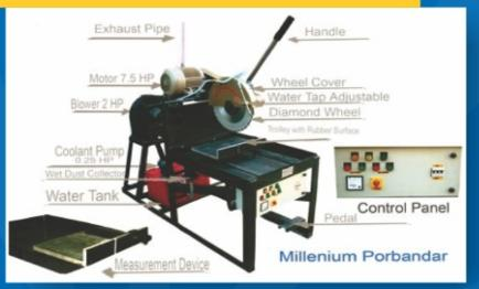
FRAME LENGTH OF BED WIDTH OF BED HEIHGT OF TABLE MS ANGEL[65/75, 06 MM THICKNESS] 39 INCH [985 MM]
