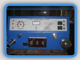
**Details:** Our instrument possesses the ability of sensing these electrical flaws in wires and cables. We are named among the eminent Manufacturers, Exporters and Suppliers of High Voltage Pinhole Tester from Maharashtra, India. The High Voltage Pinhole Tester that we offer is manufactured in adherence with the Indian Standard-13778 and IES Standard-851. Our High Voltage Pinhole Tester is stringently tested at various stages of its production in order to ensure its consistency in performance.
