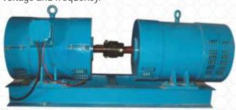
Both the above units are fitted on a common platform and coupled each other by belts drive. The three phase input to the prime mover has to be give through a suitable starter. The input to the generating unit is to be given through a variable voltage source (external) of appropriate capacity. The out can be taken from the generating unit.
