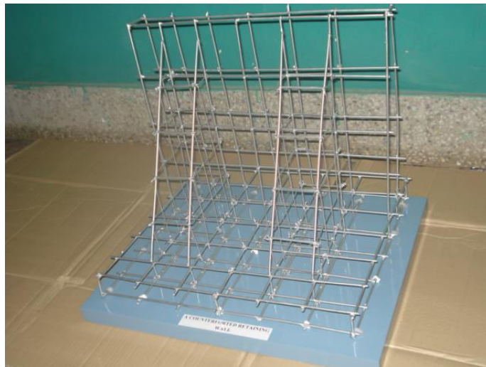
Re-Inforcement in Counterforted Retaining Wall
