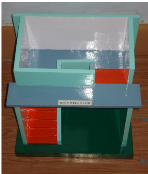
Open Well Stair Case
