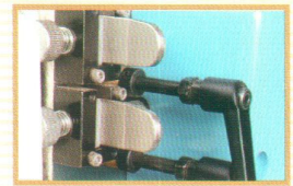
Gap setting adjustment by calipers
