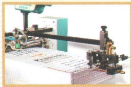
High speed flat pile vacuum feeder with back separator
