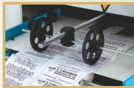
A creasing and perforation attachment at the delivery end
