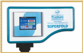
Rightly located display panel indicates information about batch counts and productivity of an ongoing job
