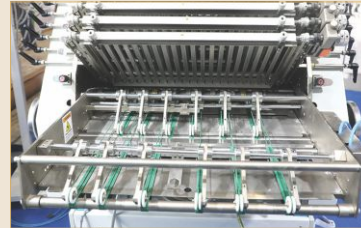
Transfer Unit with Ejection for Wrong Pharma Code.
