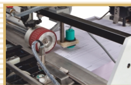
Electronic Double Sheet Detector
