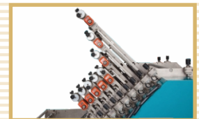
Folding Pocket with Position Indicator
