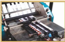
Automatic vacuum feeder feeds a single paper at a time
