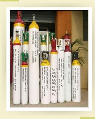
Calibration Gas Mixture - more emphatically a degree of measurement – is our prime product. Gravimetric filling method as per ISO 6142 where the components are added sequentially using traceable weights and improvised manometer method as per ISO 6146 are followed. For Analysis, various GC method and direct analysis methods as per IS, ISO and ASTM standards are used in the laboratory.
