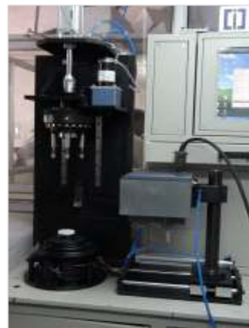
Brakedrum Gauging Station
