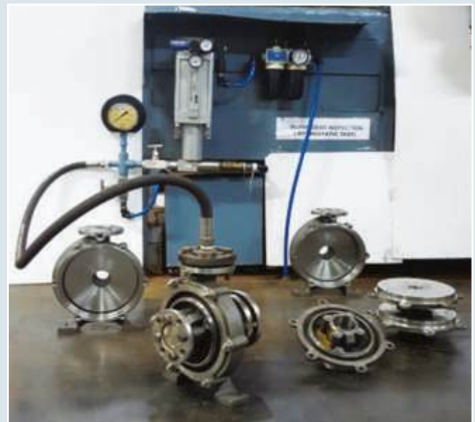
HYDRO TEST BENCH
