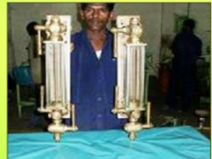
004 Boiler Gauge Cocks
