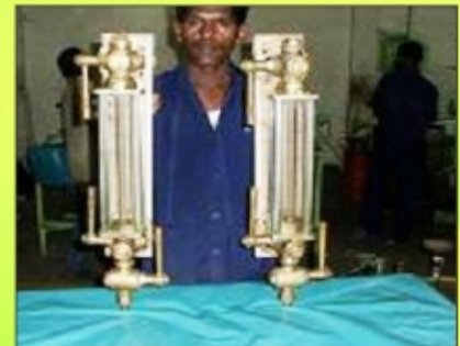
004 Boiler Gauge Cocks
