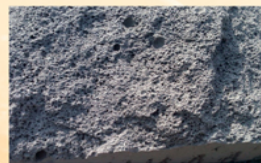
AAC cell Structure with Cavities
